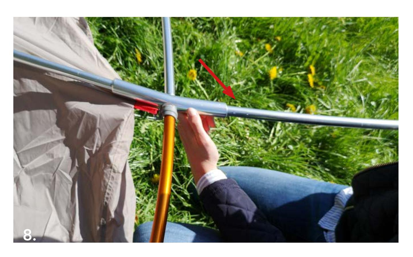
Put the two short beams together and into the other side of the connector (pic. 8).
