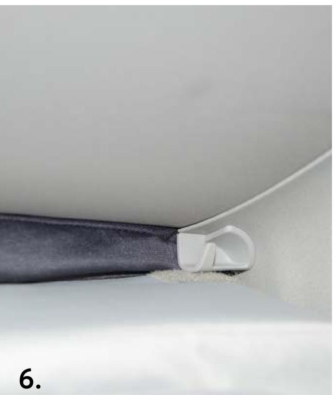
Instead of the "missing" front sun blind hook, plug the Z-angles between lining and window (pic. 5).
