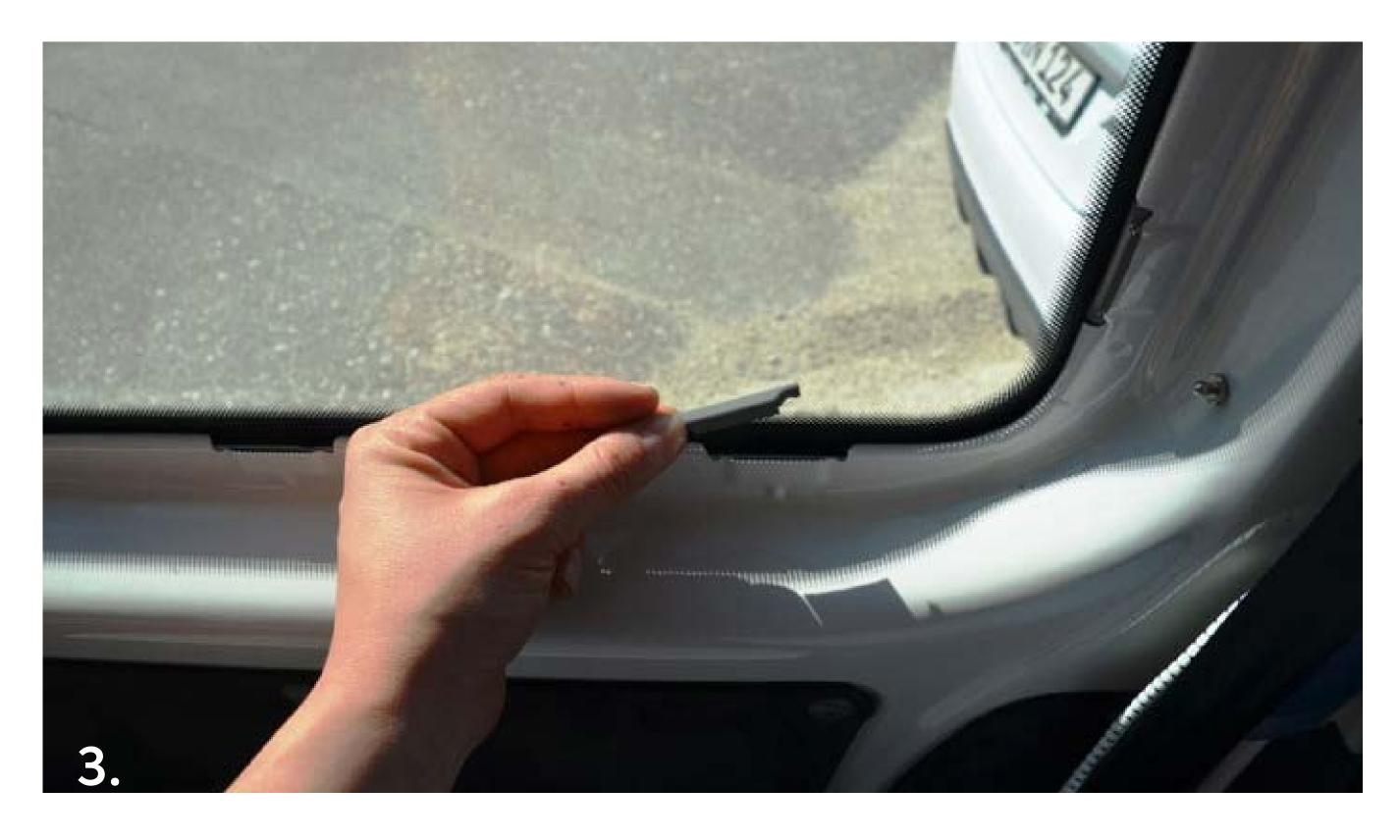
Remove the left- and rightmost plug from the lower tin lining (pic. 3).
