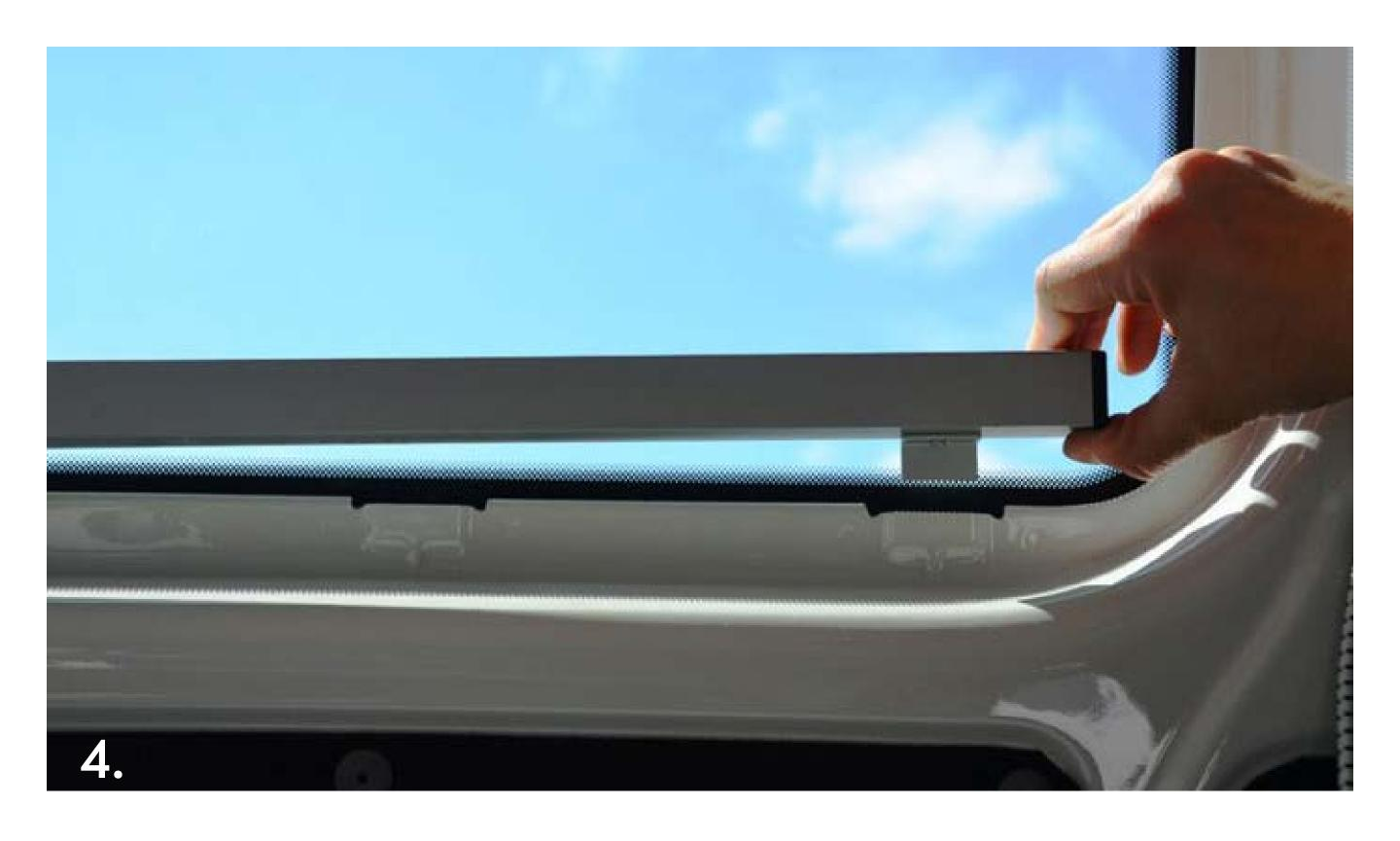
Push the angles of the aluminium bars into the aperture of the tin lining (pic. 4).
