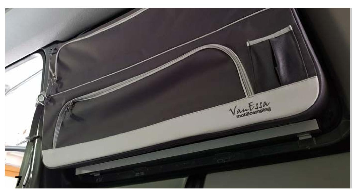
Then thread the rear panel of the packing bags behind the Z-angles (pic. 6) and push them onto the aluminium bars and completely into the window slot (pic. 7).
