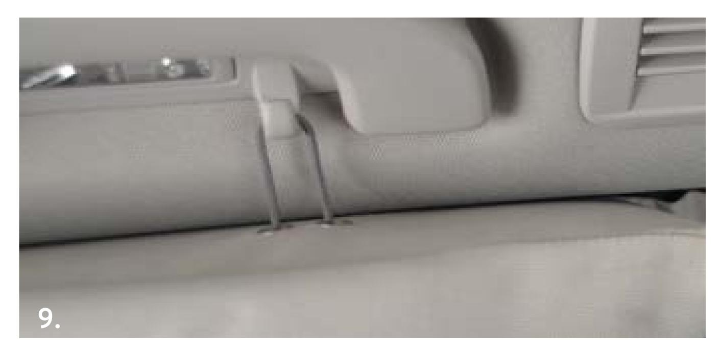
As an aditional tilt prevention, you can fix the cord on the hook under the handhold. open the zipper of If neccessery, you can open the upper compartment and push the bag a little upwards (pic. 9).
