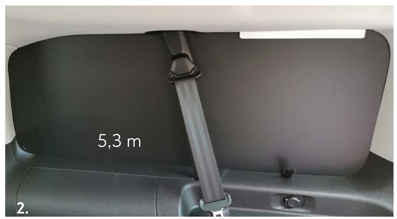
Slide the darking plate between the lining and the window (pic. 1 + 2).
