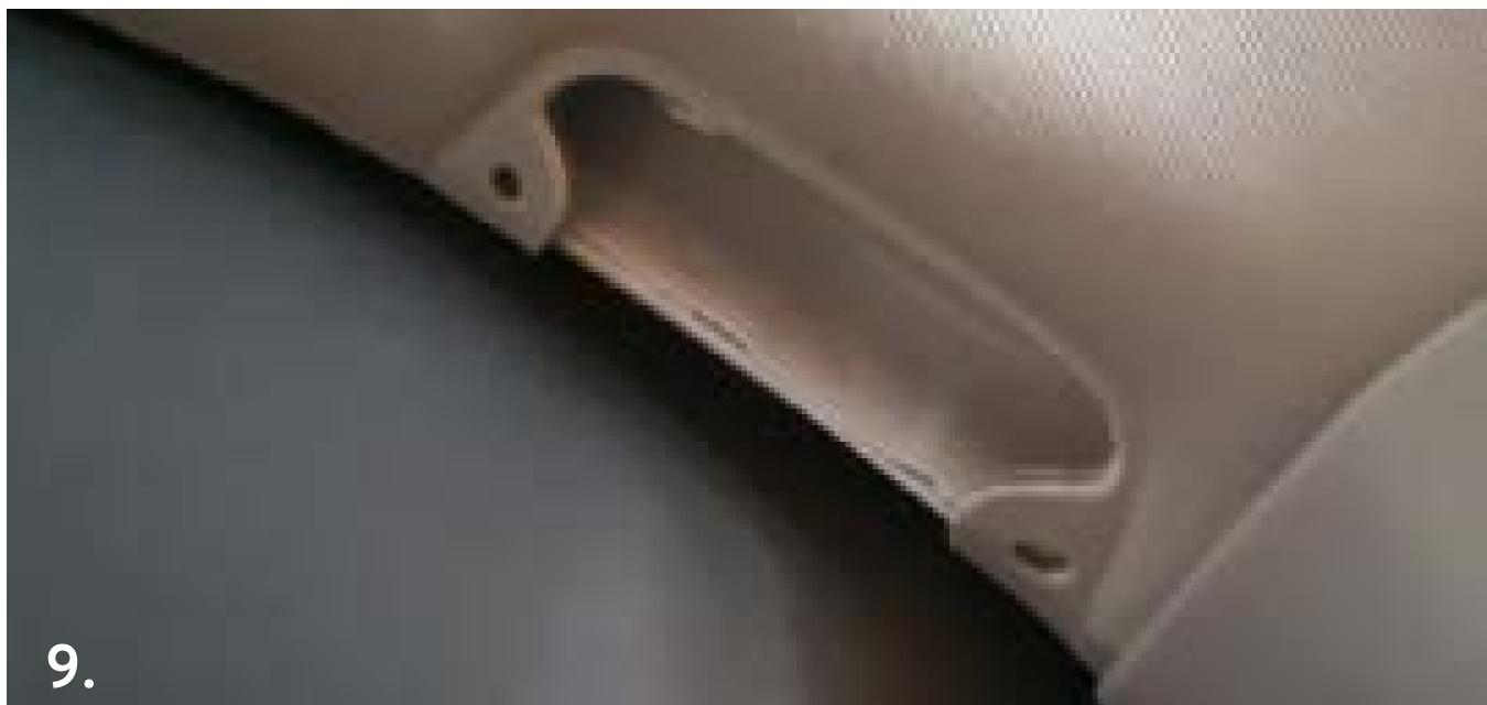
The vehicle length of 4.9 m with business equipment has a cover on each window (Fig. 8). It is possible that this is too close to the window so that the rear panel does not fit into the window. In this case, the cover would have to be removed (pic. 9).
