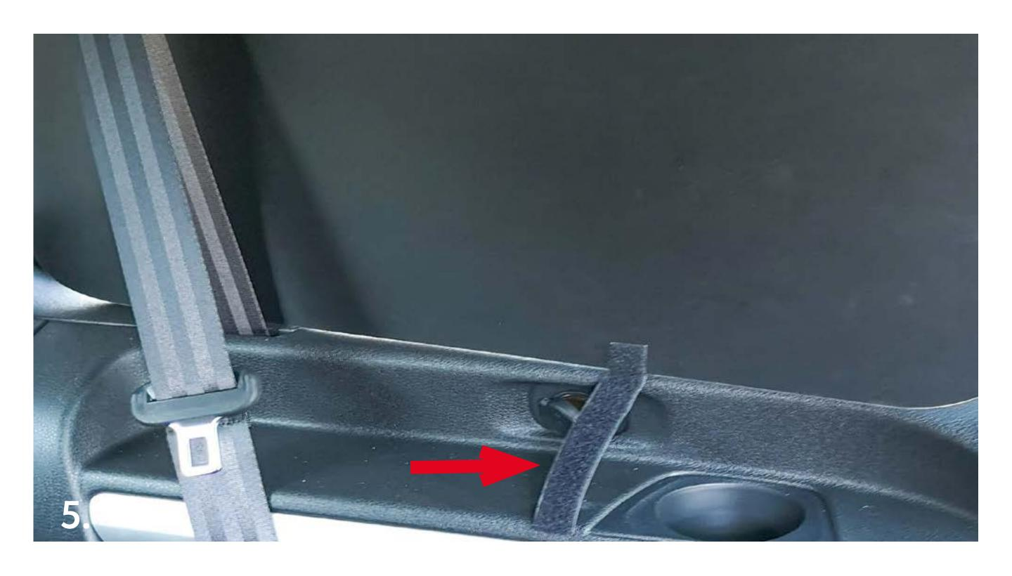
The Velcro strap (red arrow, pic. 2) has two functions. It is used to remove the darkening plate and to prevent the packing bag, which also has Velcro at the bottom, from falling out.
