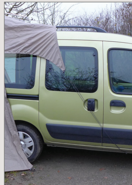
Fixiermöglichkeiten der Abspannleine am Auto Fixation possibility of the guyline at the car
