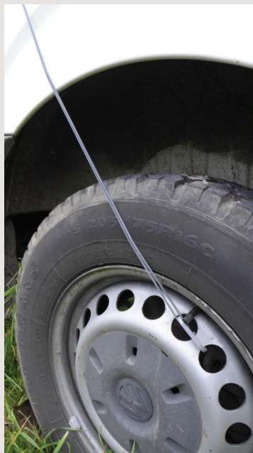
Fixiermöglichkeiten der Abspannleine am Auto Fixation possibility of the guyline at the car
