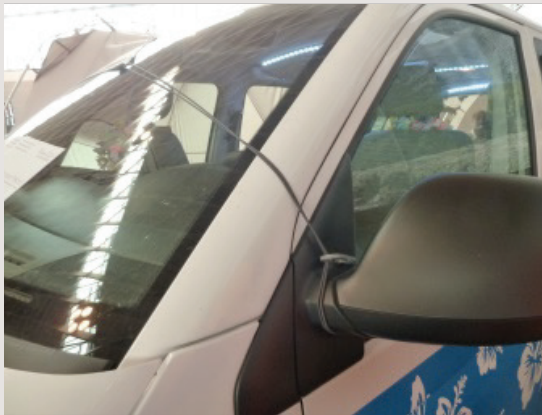
Fixiermöglichkeiten der Abspannleine am Auto Fixation possibility of the guyline at the car
